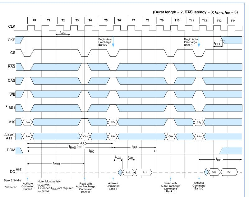
AC Parameters for Read Timing (3/3/3)
