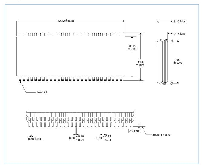
Package Dimensions (400mil; 54 lead; 2 High Stack; Thin Small Outline J Lead Package)
